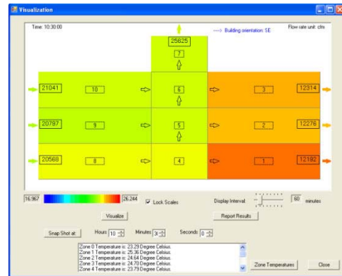
Figure 4 Visualization of results: a chromatic scale indicates the temperature of each zone and the air flow; arrows represent the direction of the flow; black rectangles show ventilation rates (cfm).
