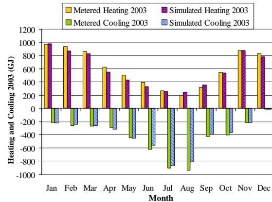
Figure 2: Metered and simulated monthly heating and cooling energy uses for 2003
