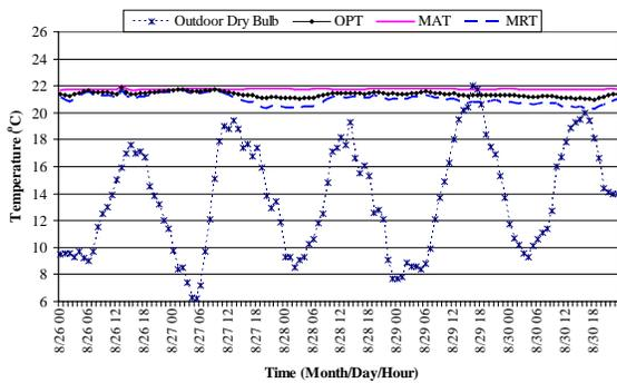
Figure 7: Measured temperature trends in an interior computer lab
