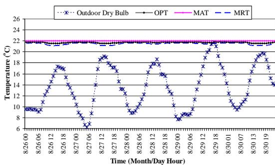
Figure 8: Simulated core zone temperature trends
