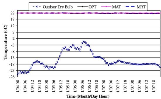
Figure 12: Simulated core zone temperature trends
