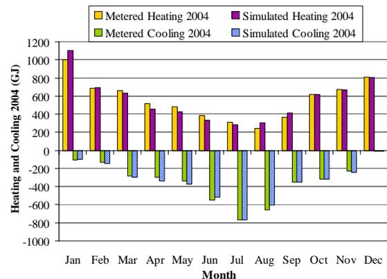
Figure 3: Metered and simulated monthly heating and cooling energy uses for 2004
