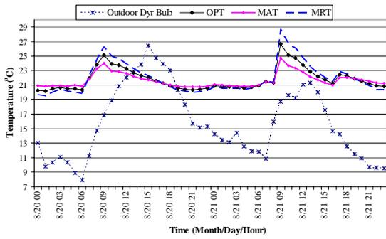
Figure 5: Measured temperature trends in an east side private office
