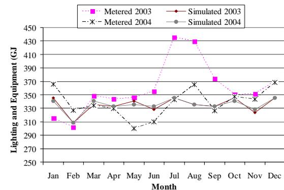
Figure 4: Metered and simulated monthly electricity uses for lighting and equipment in 2003 and 2004.
