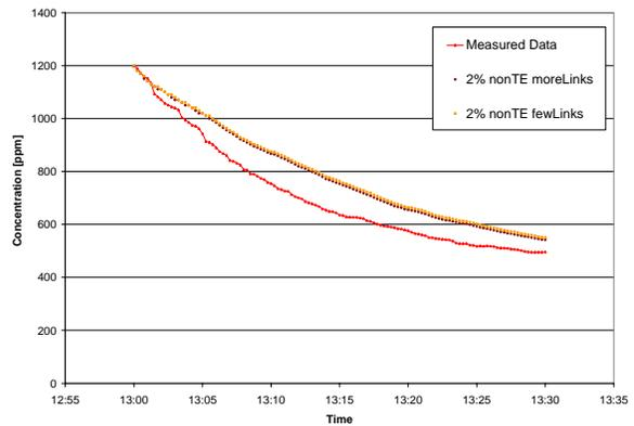
Figure 14: Sensitivity to Adding Secondary Flow Paths
