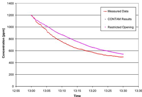
Figure 13: Verification of Flow Restriction Assumption in Experiment 2
